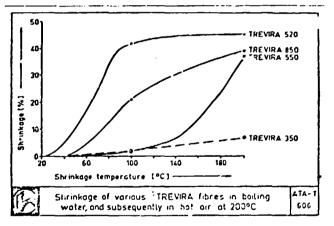
In the process of conversion from the staple fibre to the finished article, a fibre is essentially exposed to a decisive heat treatment on two occasions:
