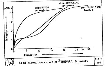
The filament possesses high strength even at low elongation and hence brings good wear properties. Woven or knitted goods made from polyester continuous filaments can be washed very easily and dry rapidly.
