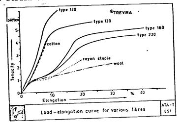
Beside the various TREVIRA types, you find cotton, rayon staple and wool. You see that, in accordance with the field of application, the load-elongation curve of the highly stretched TREVIRA 120 fibre largely matches cotton, while TREVIRA 220 is more similar to wool and rayon in its tensile-elastic behaviour, though it has a much higher fastness.
