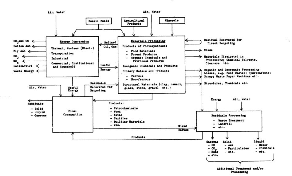
FIGURE 1: SCHEMATIC DEPICTION OF MATERIALS FLOW
