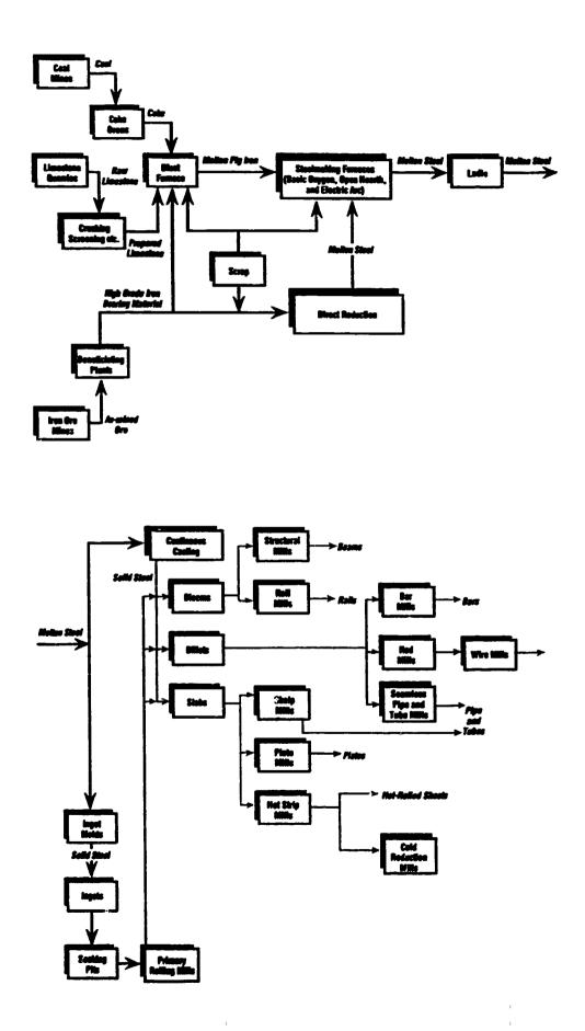
Figure 1-1 Steel Production Flow Chart
