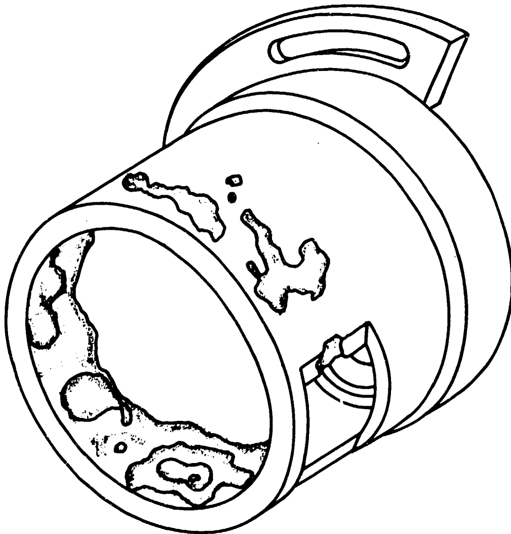
Fig. 7.3. Control cage for centrifugal shot blast machine. Note traces of wear on the internal and external surfaces and on the shot outlet hole
