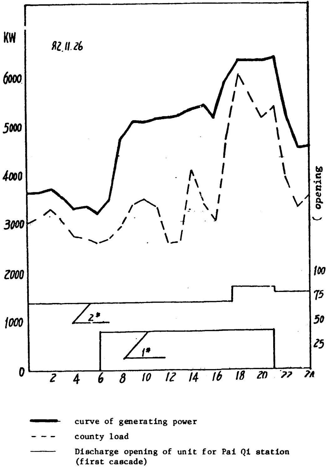
Graph 6: Operating daily load curve for paralleling state grid (Transmitted to state grid)
