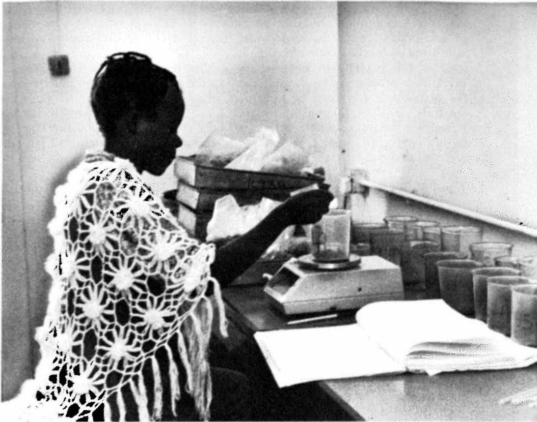
Clay tests at the Geological Survey Department, Zomba (Malawi), which are essential to the development of the country's brick and tile industry
