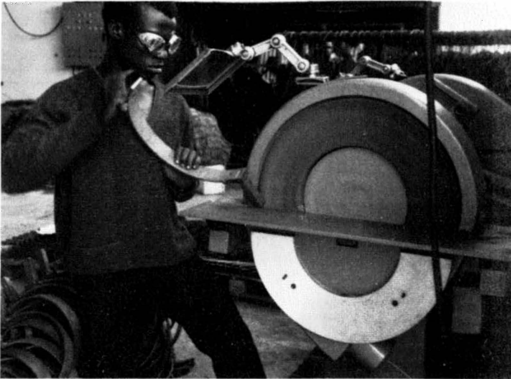
Deburring spring tines for cultivators at the agricultural implements factory UPROMA (Unité de production de matériel agricole), Kara (Togo)
