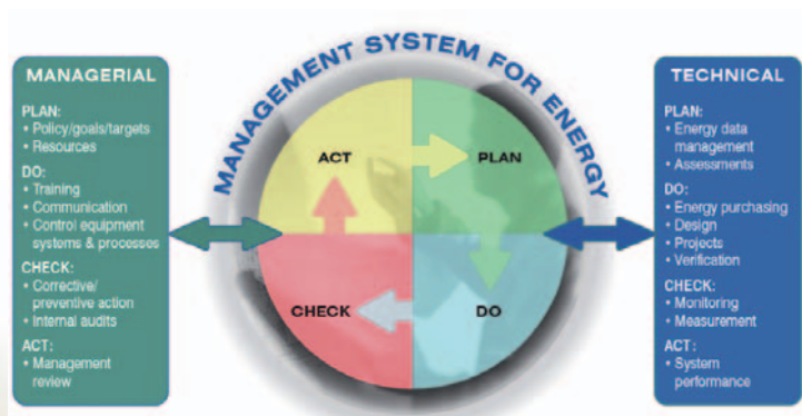
Energy management standards incorporate both management and technical aspects of energy management. Source: ANSI MSE 2000.
