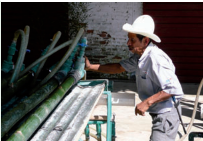
Mexican worker setting up bamboo preservation equipment
