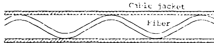
Fig.1.10: Microbends shown as repetitive changes in the radius of curvature of the fiber axis.
