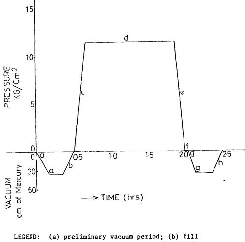
(a) preliminary vacuum period; (b) fiff cylinder with preservatives; (c) build up pressure; (d) maintain pressure level; (e) release pressure; (f) empty cylinder of preservative; (g) final vacuum period keep emptying cylinder of preservative; (h) release vacuum.
