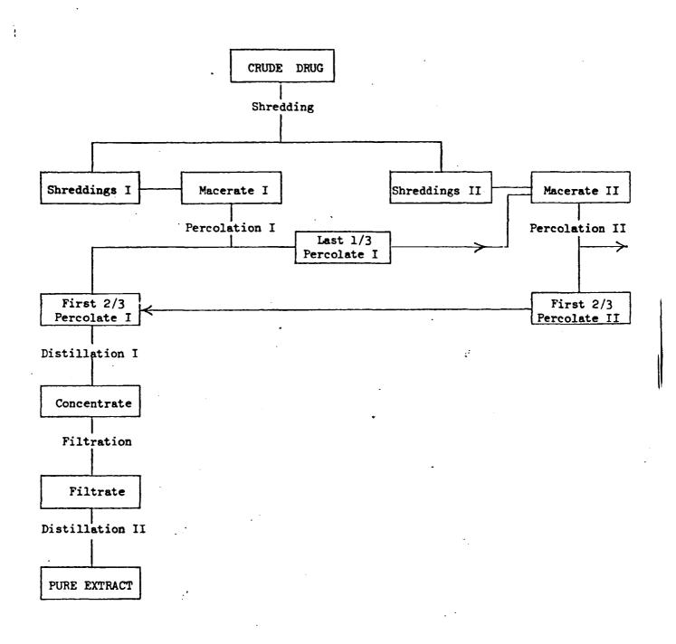
Figure IV: PROCESS FLOW: Glycyrrhiza Extract Production\_
