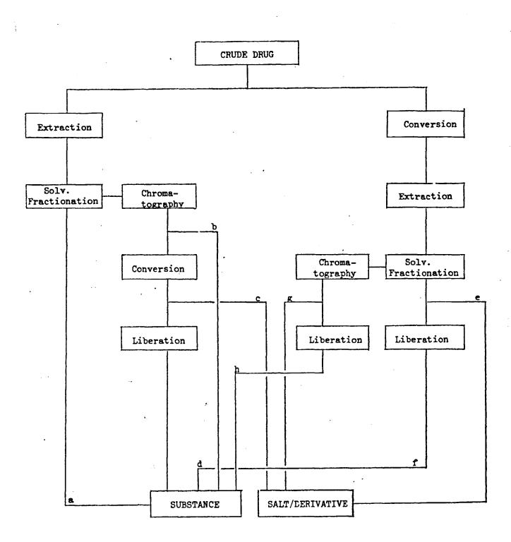
Figure V: Process Flow: Pure substances production: General scheme
