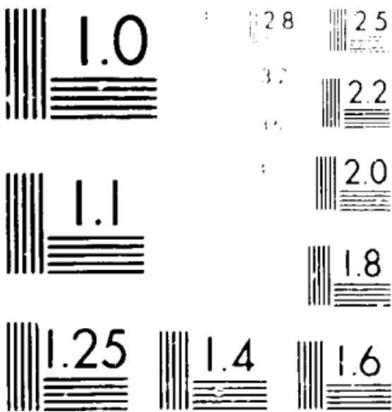
Vertical resolution of the image sensor (number of pixels per mm)
