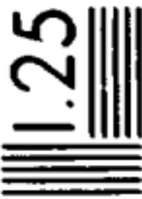
A resolution test chart for 1.25 cycles per millimeter. It consists of a central number '1.25' flanked by two groups of five horizontal lines and two groups of five vertical lines, all in black on a white background.
