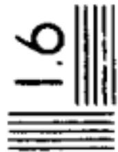
A resolution test chart for 1.6 cycles per millimeter. It consists of a central number '1.6' flanked by two groups of five horizontal lines and two groups of five vertical lines, all in black on a white background.
