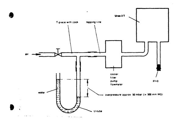
1- Close the gas outlet nipple of CO transducer
