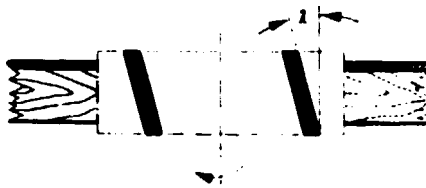
C. Cutting edges inclined in the same direction
