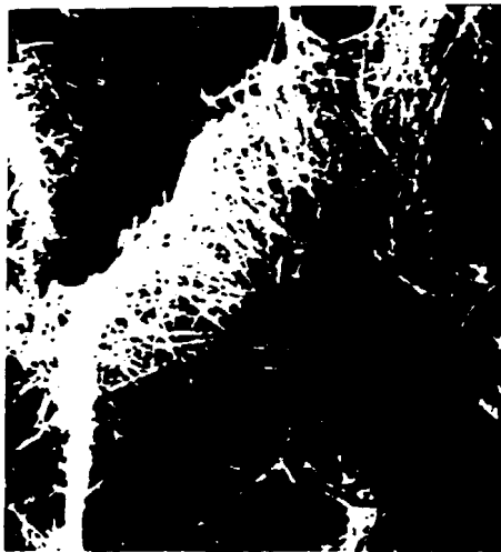
Fig. 45: The same wood, the same cement with 0.5 percent of Dextro glucose. The crystals are thin and long fibres which are not able to develop board strength. The bar represents 10 micrometres.
