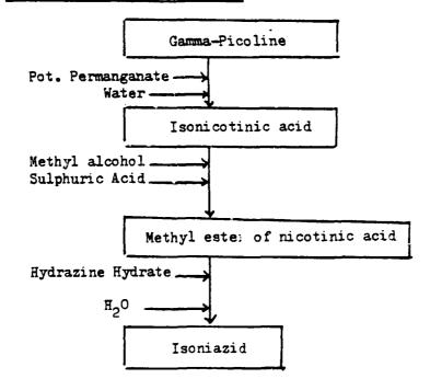
Note: In another alternative process, first step oxidation of Gamma-Picoline is carried out by mixture of Nitric acid and sulphuric acid.
