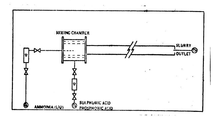
All the heat of reaction produced in neutralization of the ammonia by the acid is absorbed in the evaporation of the water present. Since the slurry formed need not be pumped, its water content, and thus its fluidity, may be much lower than in the case of the conventional processes described above. The water is eliminated in the form of vapour at the exit from the outlet tube, and since the liquid phase in the granulator is smaller it is possible:
