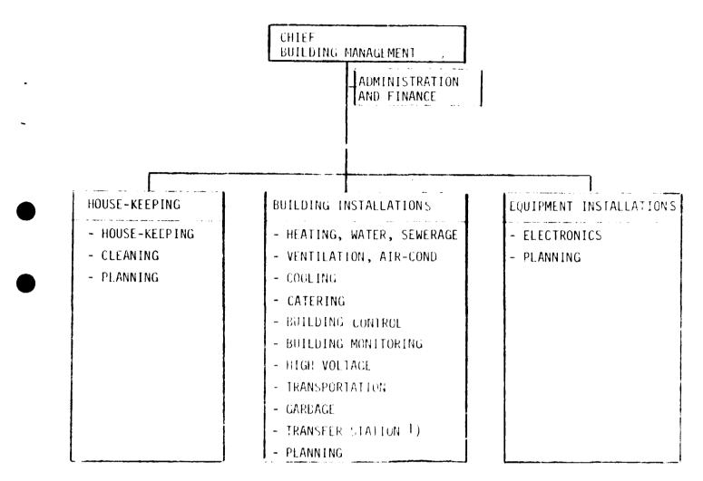
In this structure, the functions have been divided into three main groups; a house-keeping unit, a building installations unit and an equipment installations unit. All units have the total responsibility for each function and carry out all tasks (see paragraph 4:2).
