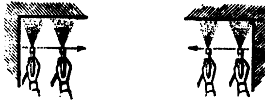
Figure 20 Correct pointing of gun at corners.
