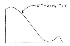
Equation for the Ogee profile for upstream face vertical  $\rightarrow X^{1.85} = 2 \times H_d^{0.85} \times Y$
