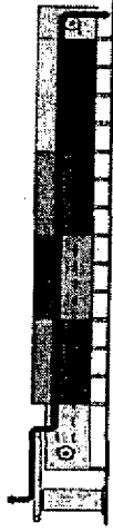
Figure 27: One-Belt Drier with alternating ventilation in the different zones of dryer (Stela 2006)
