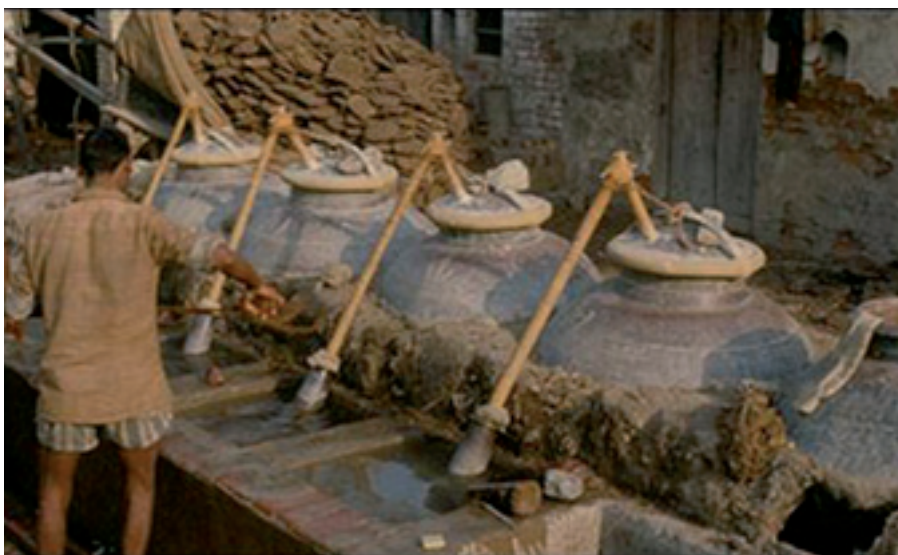
Figure 1: Traditional Indian deg bhapka method
