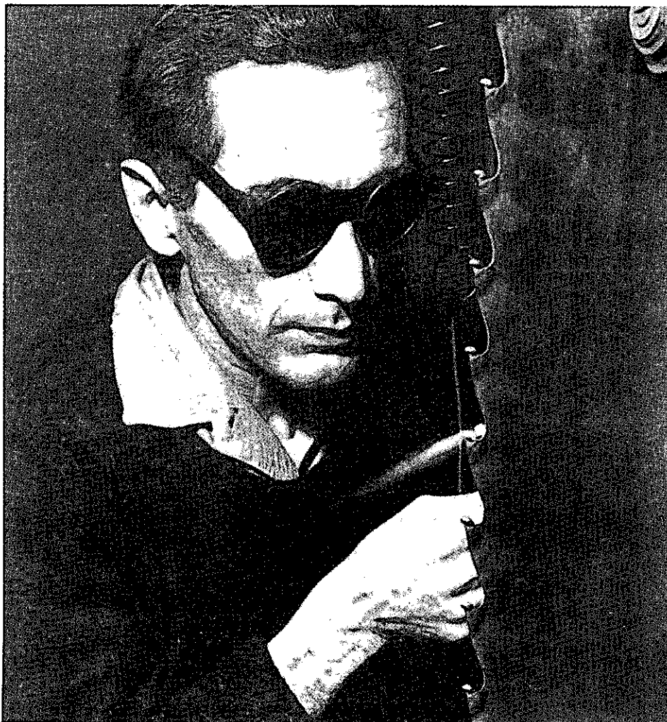
Figure 31. Blade held in such a way that teeth are pointing upward in the direction of the welding
