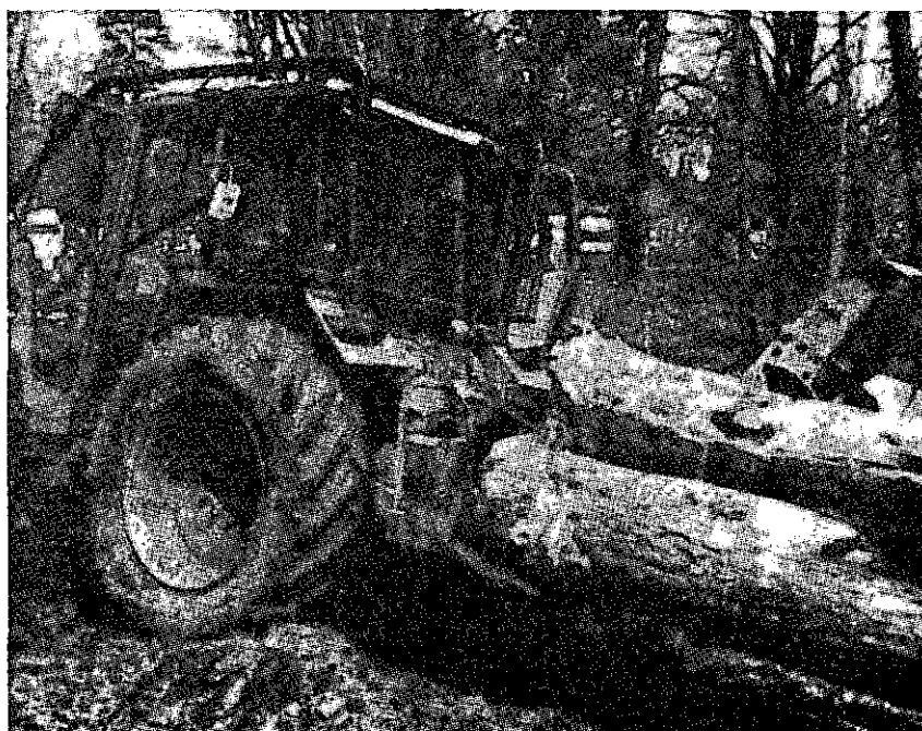
Figure 4. Two-drum winch used on a farm tractor
