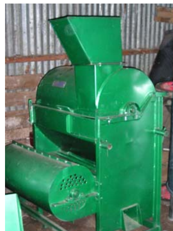
Fig .4.5 Rubber roller rice dehuller
