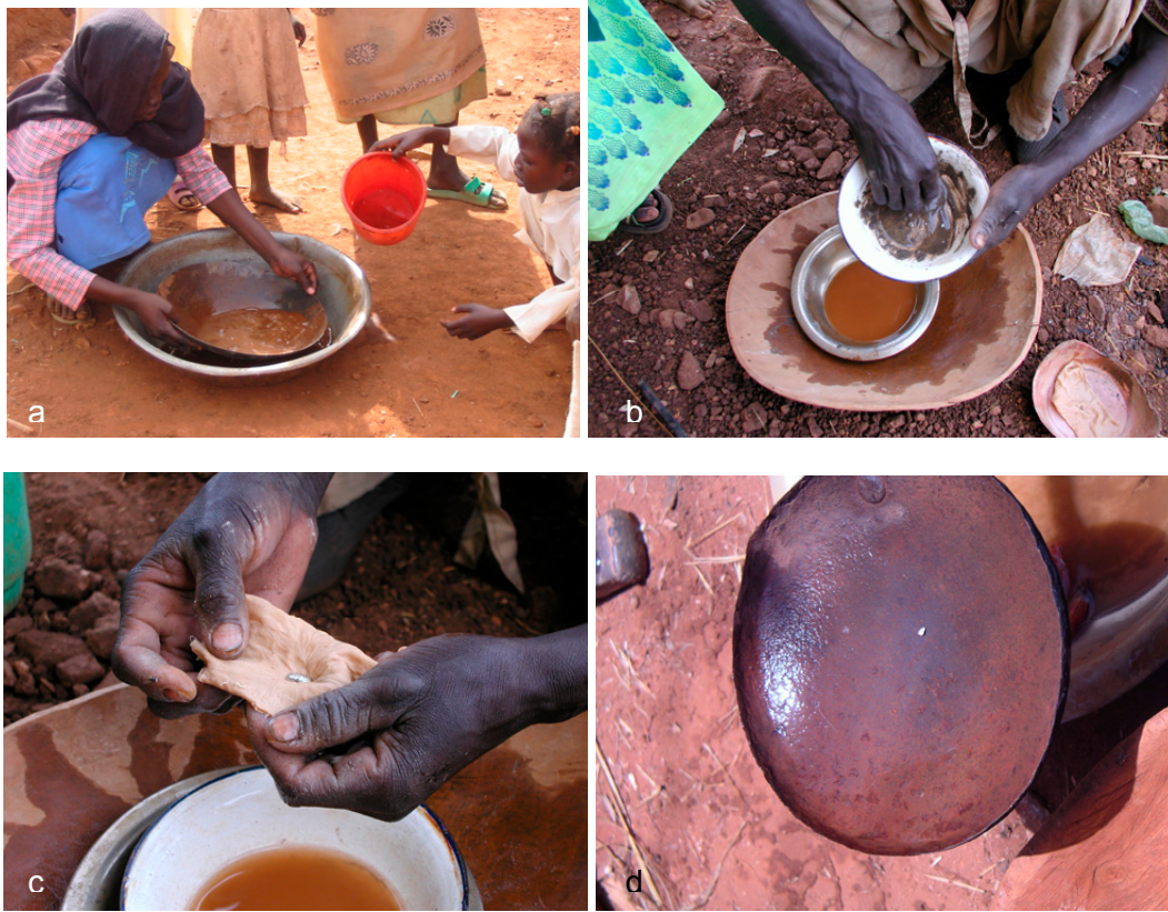
Illustration 9 - Gold recovery process phases (a) Panning; (b) Amalgamation by hand; (c) Squeezing with piece of cloth; (d) Roasting on frying pan
