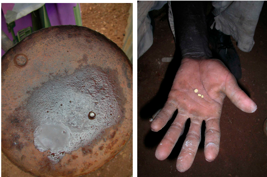
Illustration 11 - Example of amalgam before roasting (left) and “doré” (right) after roasting
