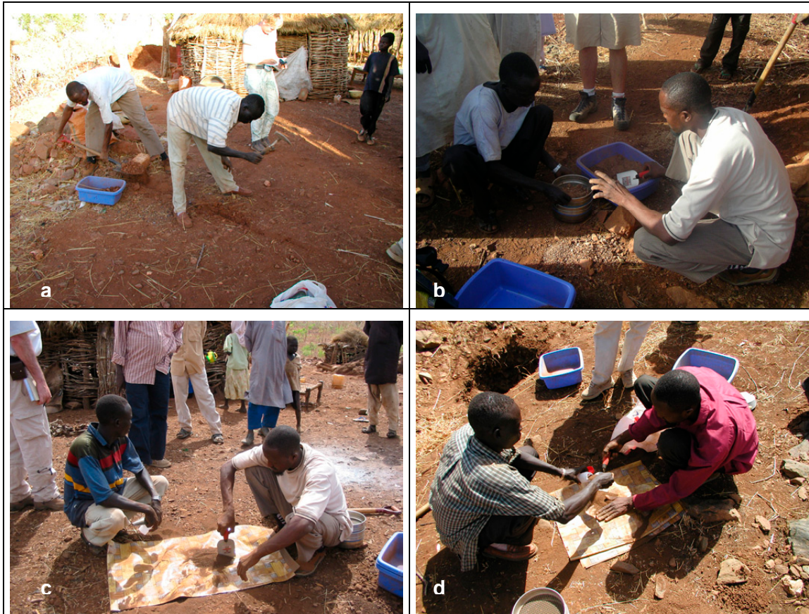
Illustration 26 - Soil sampling phases – (a) Digging along line or point; (b) Sieving; (c) Sample splitting; (d) Collection in bottles
