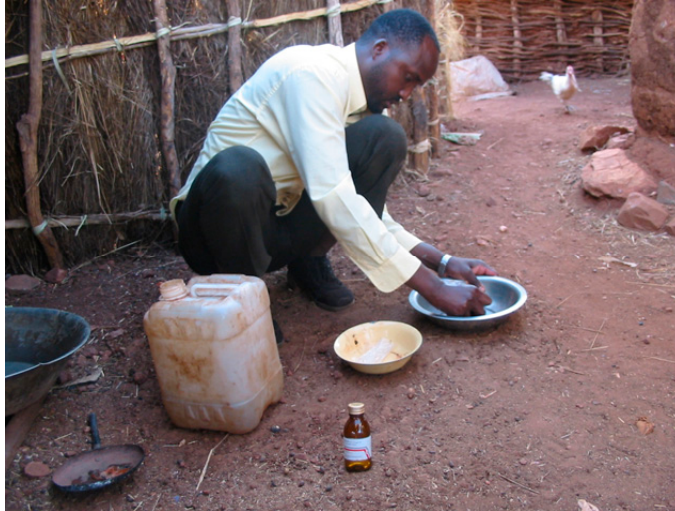
Illustration 10 - Amalgamation performed without precautions in the “family units”
