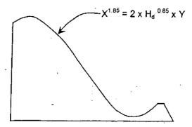
Equation for the Ogee profile for upstream face vertical  $\Rightarrow$   $\chi^{1.85}$  = 2  $\times$  H<sub>d</sub>  $^{0.85}$   $\times$  Y
