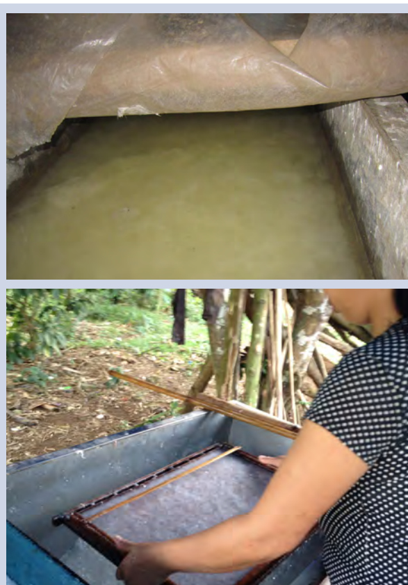
FIGURE 12: The old cement (top) and new stainless steel tanks
