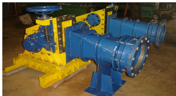
Two number 35kW SHP Turbine manufactured by Nigerians through a technology transfer partnership between UNIDO/NASENI
