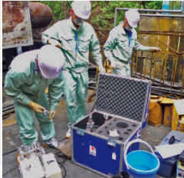
Collecting stack gas samples at a waste incinerator in Viet Nam.
