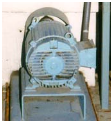
15 kW Motor Efficiency is ~ 91%
