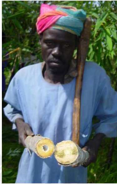
Cross section of culm showing hollow upper culm (left) and completely solid base (right)
