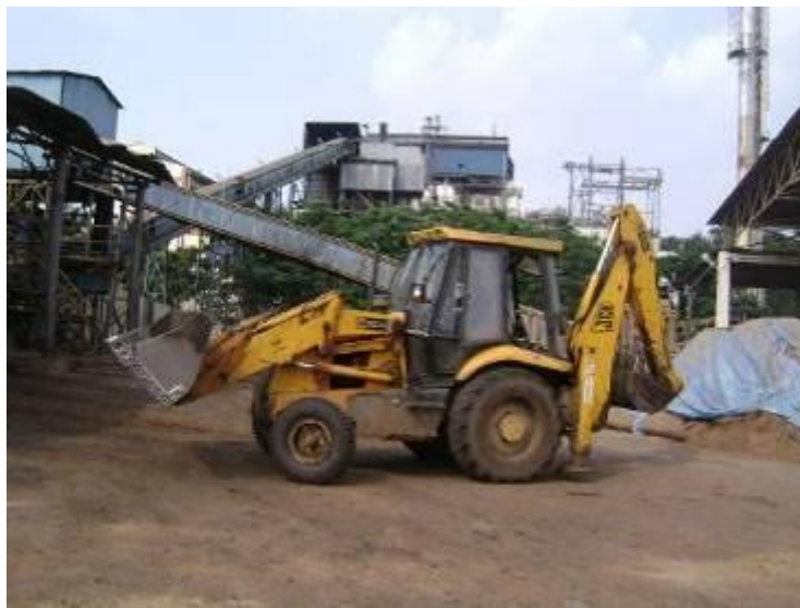
Figure 11: Typical front-end loader for fuel handling
