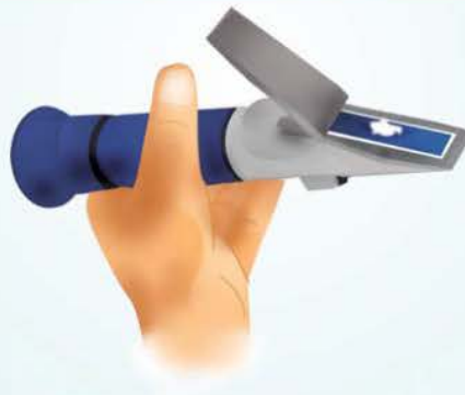
Clean the prism with distilled water and dry with a soft tissue to proceed with the next sample
