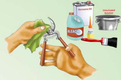
Keep a tools cleaning kit (kerosene oil, Bleach, Lubrication oil, clothe and brush)
