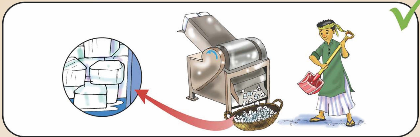
Ice crushing machine should be used to crush the ice.
