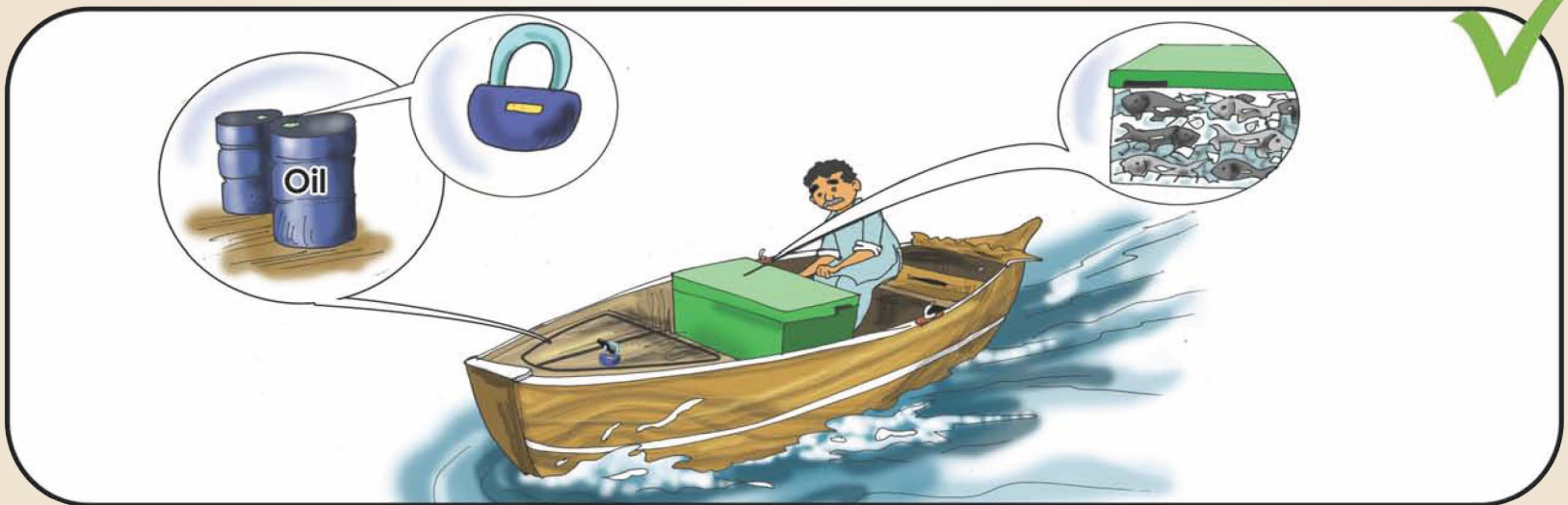
Areas with fuel and oil should be well sealed and separately stored to prevent fish contamination.
