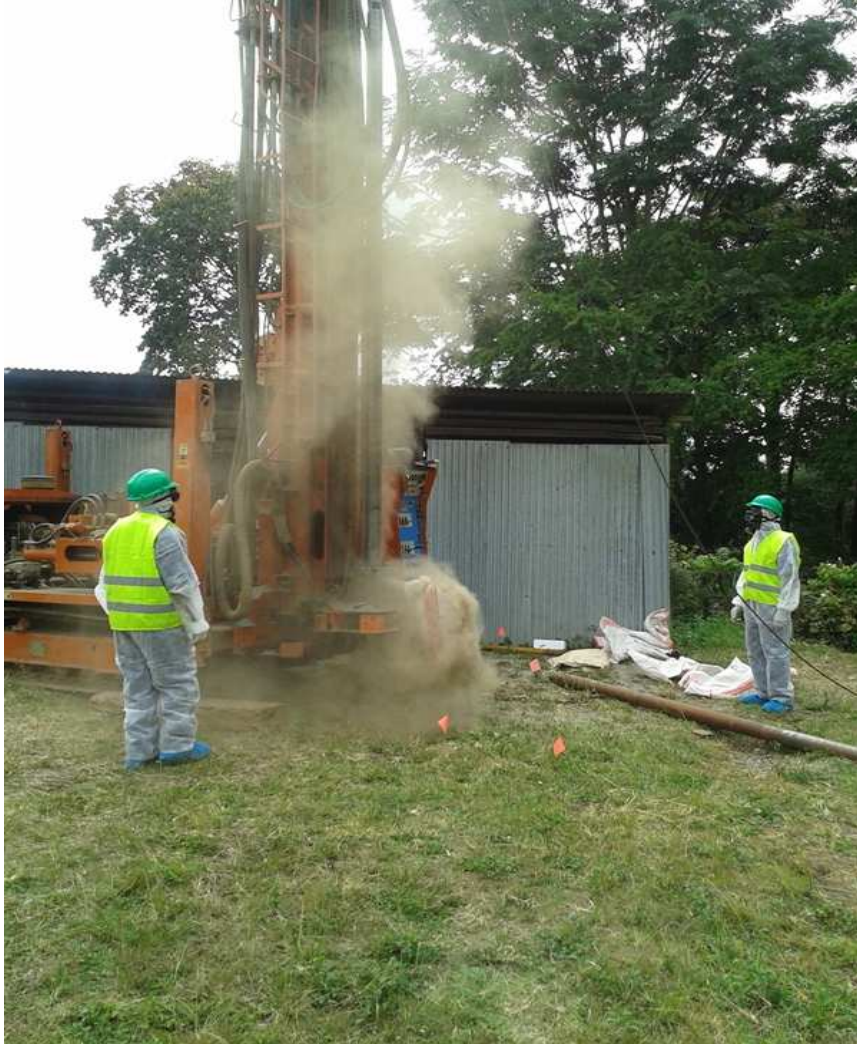
Profile core sampling- DSI
