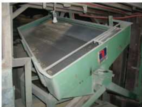
Figure 14 Paddy tray separator source: (IRRI, 2009)
