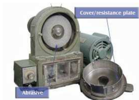
Figure 16 Abrasion machine, source: (IRRI, 2009) Friction whitening eliminates the bran via friction between the rice grains themselves; it is composed of a rotating cylinder with a metal screen as the external wall containing the brown rice.
