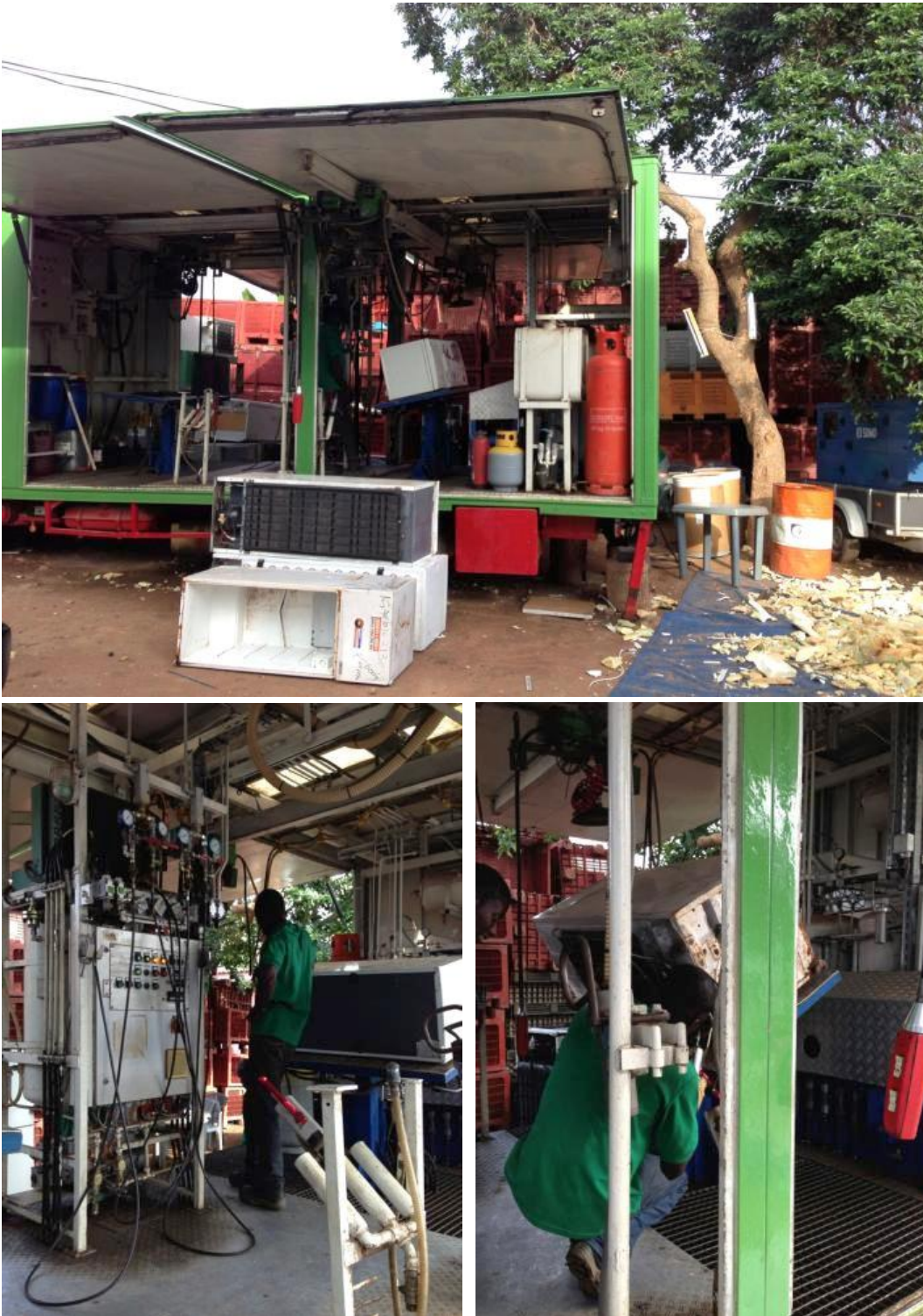
Figure 10: Formal refrigerator treatment in Ghana: mobile treatment plant for de-gassing of refrigerators (top); details on de-gassing operations (bottom left) on a refrigerator.
