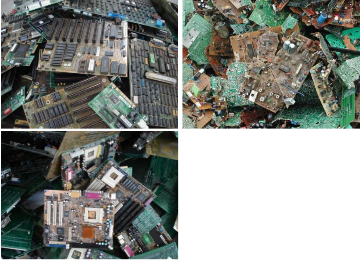
Figure 14: Low grade PWB like from consumer electronics, TVs and monitors (top left), medium grade PWB from telecommunication equipment (top right) and high grade PWB from old generation personal computers (older than Pentium IV, bottom left)
