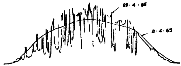
FIG. 2—Record of insolation on day of broken cloud superimposed on record for clear day at Gladstone, Queensland, latitude 28° S.
