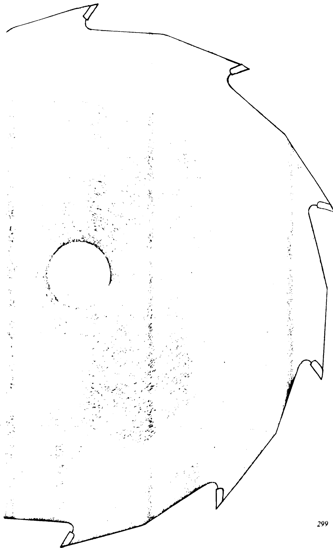
Figure III. Wide-pitch circular saw blade
