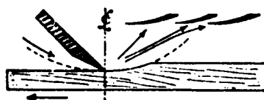
Figure IX. Action of a rotary cutter
