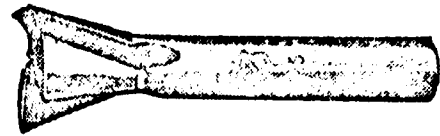
(c) With 3 cutting edges
