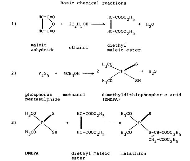
The first reaction takes place in the <u>esterification reactor</u>. The reaction mass is heated and the solvent, excess ethanol, and water distilled through a column.
