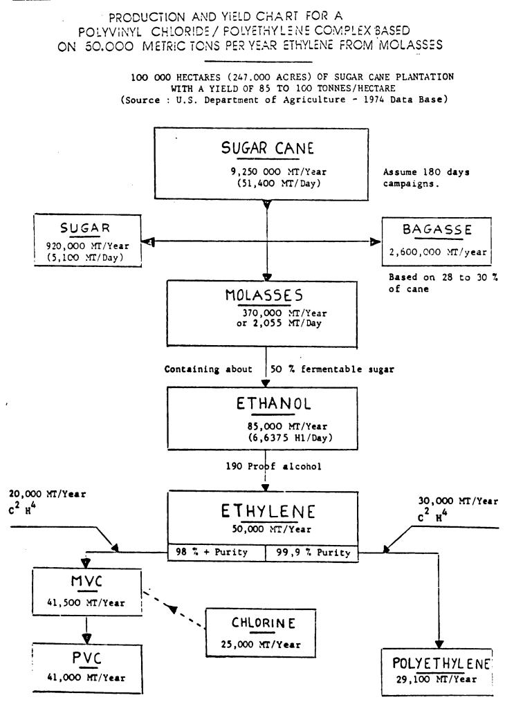
PRODUCTION AND YIELD CHART FOR A POLYVINYL CHLORIDE / POLYETHYLENE COMPLEX BASED ON 50000 METRIC TONS PER YEAR ETHYLENE FROM SUGAR CANE
