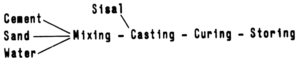
FIG 6.1. Material flow using chopped fibres.
