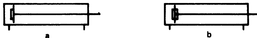
Figure 39. Double-acting cylinders with cushioning at (a) one end and (b) both ends
