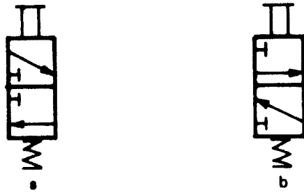
Figure 58. Alternative symbols for the two-position, three-port valve
