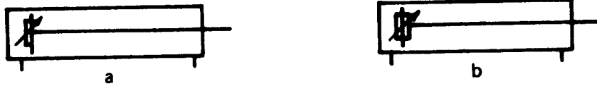
Figure 40. Double-acting cylinders with adjustable cushioning in (a) one end and (b) both ends
