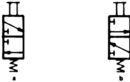
Figure 60. Alternative symbols for the two-position, three-port valve
