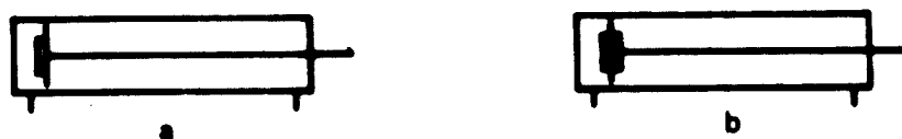
Figure 39. Double-acting cylinders with cushioning at (a) one end and (b) both ends
