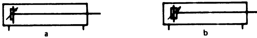
Figure 40. Double-acting cylinders with adjustable cushioning in (a) one end and (b) both ends
