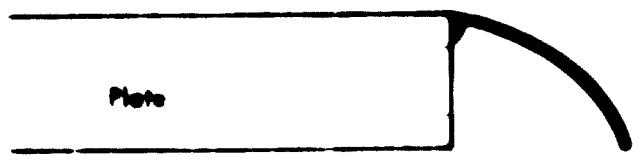
I Sheet metal welded on to
