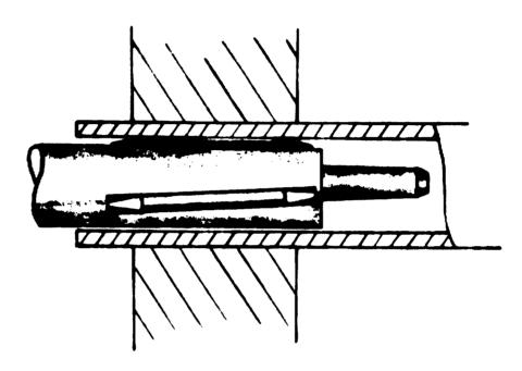
For tubes that extend beyond the open face of the tubesheet, a thrust collar that fits over the tube must be used. The thrust collar positioned against the tubesheet face will accurately locate the expanding rolls within the tubesheet hole. (Fig. 2)
