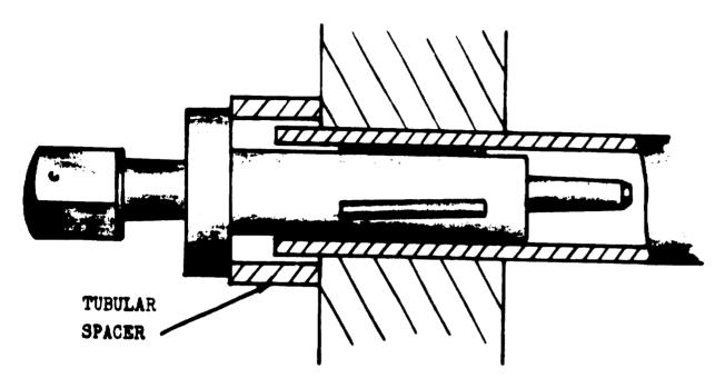
It is important that free expansion beyond the tubesheet be avoided. Belling or flaring of the tube ends is not recommended. However, if this operation is necessary, proper rolling techniques for the particular tube size will be furnished by Alan.
