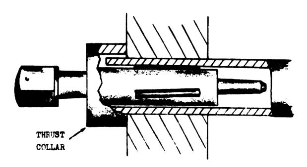
If the expander is not equipped with thrust coilar (Fig. 3), a tubular spacer may be improvised with an inside dimension sufficient to accept the tube ends and with a proper length to place rolls accurately within the tubesheet hole.
