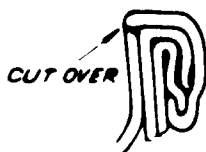
Figure 23. Double seam at lap cross-section
