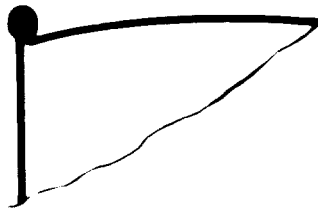
Figure 27. Welded seam used for connecting top and bottom covers to the shell of heavier steel drums
